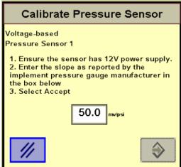
check valves. In that case, simply unplug the sensor while this setup is being done so it will calibrate the zero point correctly.
