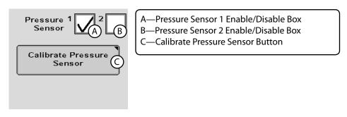
**4.** To calibrate pressure sensor(s), select button (C) and follow on screen instructions. See Test section (GreenStar™ Rate Controller Manual) for details.
