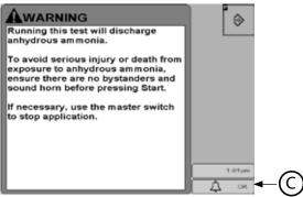
**4.** Turn vehicle into the wind. Turn on Main Master Switch on console. (Master Indicator at lower center of screen (D) will change to Master On). Press Override Height Switch (E) to temporarily disable the implement height sensor. Press Start (F). Repeat as needed to prepare system for fieldwork. If needed, turn Main Master Switch off to stop flow immediately. Return to Setup or Main menu.
